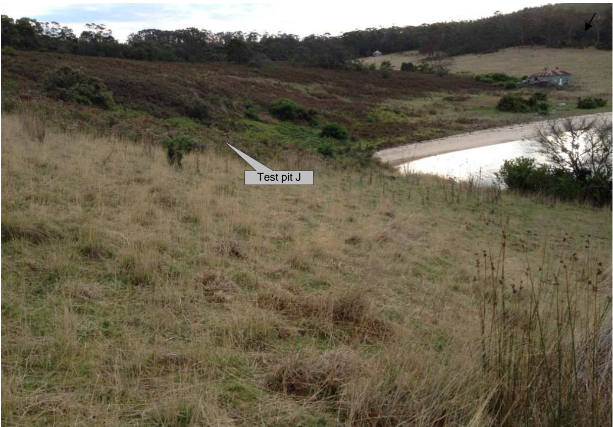
Plate 8 (below). View NNE towards test pit J. The hillside shown here is composed of Quaternary-age colluvial deposits of silty gravelly clay and clayey sand up to about 2m thick overlying Permian-age siltstone.
