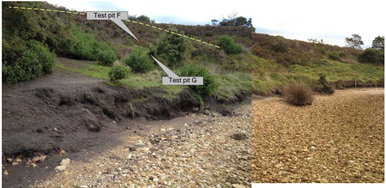
Plate 5 (above). View north towards test pits F and G. Siltstone bedrock was present in the base of test pit F at 2m, and beach shingle similar to that in the foreground was exposed in test pit G at 1.6m. The yellow dashed line is the (very approximate) northeastern limit of a probable shallow translational landslide in aeolian sand and silty sand. The dark-coloured silty sand soil is (a) probably moving downslope very slowly, and (b), is being removed at about the same rate by marine erosion.
